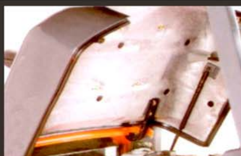
The Sound-absorbed Materials - Heat-insulation/vibration absorbing - Lowest noise - Rubber sealing packing at the gap between engine hood and truck body
